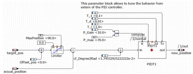
Figure 3: Modelling CA using ASCET block diagram editor [17]
