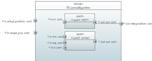
Figure 2: Modelling the structures of CA using IBD [17]
