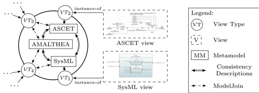
Figure 1: The modular SUM Metamodel concept of Vitruvius at the example of automotive systems engineering from [17]
