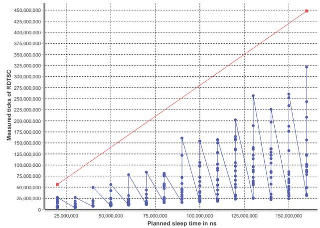
**Figure 1: TSC is not dependable: Zigzagged blue line shows the relation between requested sleep times (x-axis, in ns) and values measured with TSC (y-axis, in CPU ticks; 1 tick = 1/2.8 ns); straight red line shows the number of CPU cycles (y-axis) corresponding to the requested sleep time (x-axis)**
